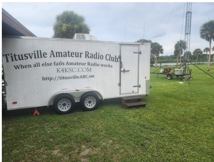
This is TARC-1, our portable operating station. Field Day checks out all of its operating functions and provides an operational base for any communications needed for public service, disaster, or backup communications that might be needed by any group, agency or organization. It's equipped with three (3) HF radios, two VHF/UHF radios, air conditioning and comfortable operating positions with computers ready to support. It is the result of quite a lot of work by TARC members past and present, and is ready to support when needed.
