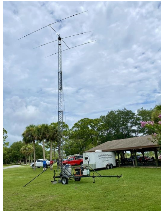
Here is the portable antenna trailer with mast extended, and Cushcraft A3S multi-band beam antenna on top. Generator provides AC power. It also supports a multi-band dipole. If you haven't seen this trailer in operation, you're missing out on a very cool piece of critical equipment.
